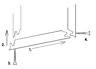
Please note the correct assembly of the easy interlocking joint shown to the left. The screws or nails MUST be installed only in the edges shown (3 & 4). Installing on the other edges will result in open seams. (Pre-drill if using screws.).
