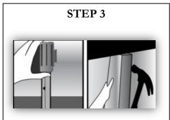
Raise the soffit slightly and install a brace so that the opening is slightly increased for easy installation of column.
