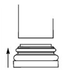
1. The shaft of an *Architectural PolyStone* \*column is designed to sit on top of this base. This base must be included in your overall height when cutting the shaft to required length. Use a fiberglass epoxy to adhere base to shaft. (For regular PolyStone\* columns, the base slides over the bottom of shaft and does not add height.)
