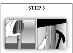
Raise the soffit slightly and install a brace so that the opening is slightly increased for easy installation of column.
