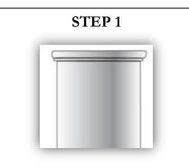
Before installing the decorative capital, cut the column at the top of the shaft just above the astragal (neck bead) within 1/8" from the astragal & belt sand flush to finish. (Skip this step if the columns were ordered "cut at bead" from the factory) STEP 2
