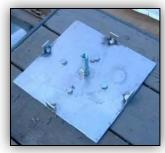
Note: Deck plates must be bolted to the top of the wood or composite deck with four (4) ½" stainless steel lag bolts. 2" x 4" Blocking must also be used on the underside of the deck for extra support. (The ½" bolts are sold separately).
