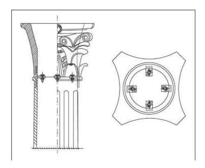
Decorative PolyComposite capitals include imbedded brackets for easy installation and to ensure load-bearing capacity. **Standard:** Above is standard for 18" and larger. **Add-On:** Above may be applied for 16" and below for an upcharge.
