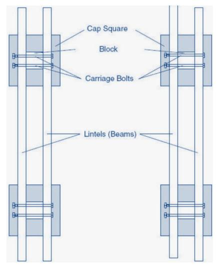
\*\*\* Note: Depending on the type of bracket used, these can be installed prior to cap and block installation to give more room to make connections. These brackets only help to prevent twisting and are not designed to be the structural attachment. That is the purpose of the threaded rod. \*\*\* Once the block is attached to the column and aligned, finish tightening the threaded rod.
