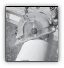
Use an abrasive saw (masonry or carbide tip blade). Fine trim top and bottom with rasp to assure flat surface contact.
