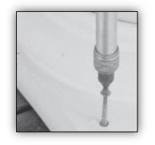
Apply construction adhesive to bottom of base and nail or screw to floor. Use a non-acetone based exterior grade construction adhesive.
