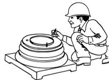
Pre-drill holes at top of base molding. Place headless nails (blunt side down) into holes. If additional holes are desired, use a steel cutting drill bit. Headless nails can be made by cutting off galvanized nails.
