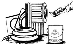
If the column shafts are trimmed to different lengths, the bottom end grain must be sealed and painted with a waterproofer or wood preservative and painted with an exterior oil-based paint to help prevent moisture related cracks and premature decay or rot.
